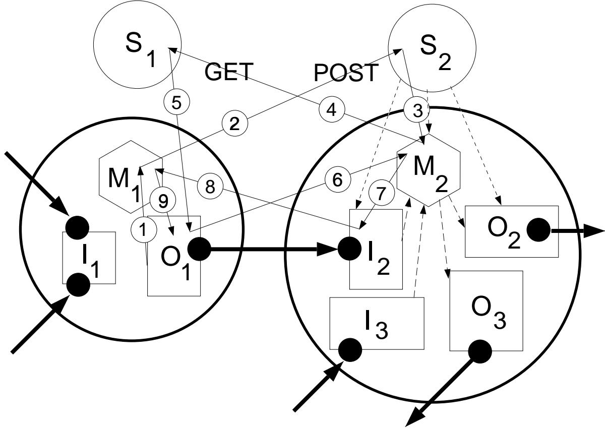
**Figure 1** This diagram illustrates point-to-point communication between Web servers, used to implement a webflow channel between compute-web modules. Two extreme implementation modes are described: a) based on today's Web server technology, and b) based on thread memory mapped high performance implementation, expected in future Web compute-servers. Subsequent steps, represented by a sequence of labelled lines in the figure, are described below in both implementation modes.
